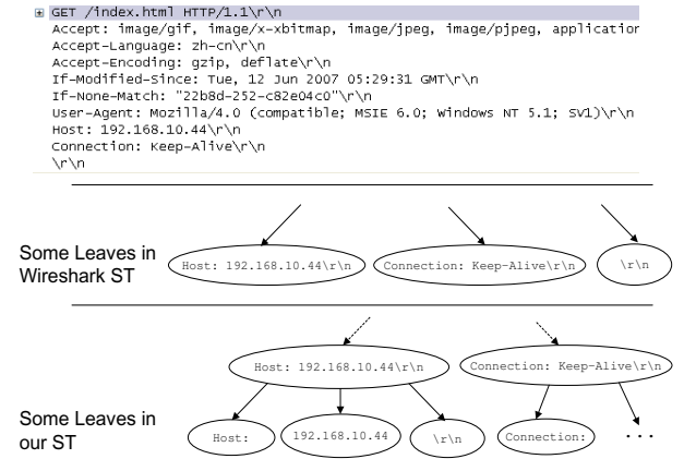
Wireshark Formated Data (an HTTP GET Request)
